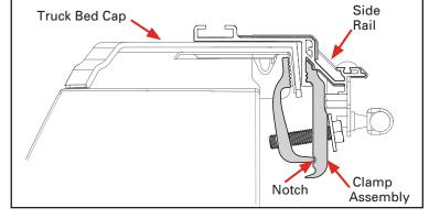
Attach one clamp (O) from the passenger side rail (B) to the truck bed. Disassemble the stake pocket clamp (O). Place the inner part of the clamp into the rail. Make sure the bolt passes through the stake pocket hole as shown.
