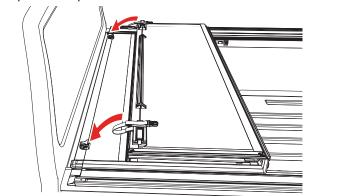
FLIPPED UP POSITION: Fold the cover (C) open and lift it until it's vertical or past 90 degrees towards the truck cab. Then release the prop rod that is attached to the rail. Fold the prop rod over and position it firmly against the vertical plate on the underside of the cover. Then slide the prop rod locks downwards and tighten the knobs to lock it into position. Do this on both sides of the cover. The cover should be firmly in position with little to no movement once the prop rods are locked.
